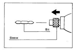
To remove the bit, pull the sleeve in the direction of the arrow and pull the bit out firmly.
